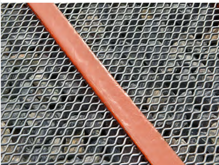
Square self-cleaning screen with polyurethane bands
